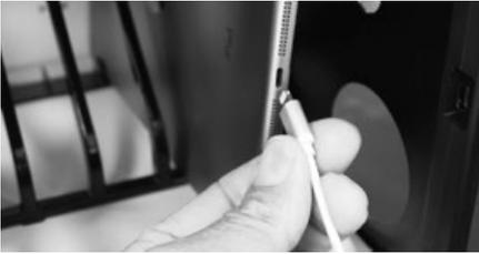
Plug in the power cord, connect to a wall outlet and switch it on. Charging will automatically start.
