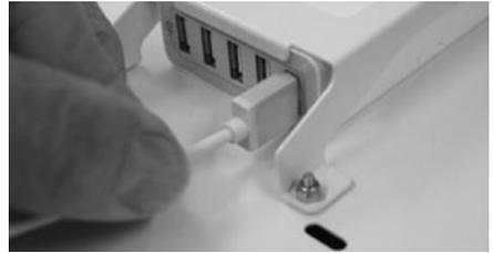
*NOTE: Use the green velcro cable ties supplied to neaten the cables if using long cables.*
