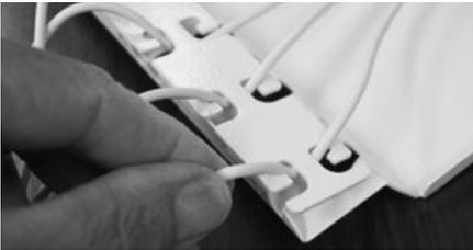
Route the cables through the 'tear-drop' slots.
